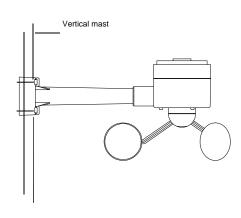
Check that the wind-cups can rotate freely before fixing the unit. For correct and accurate readings, it is important to mount the sensor with the cups on the bottom. The wind sensor should now be mounted using the screw or cable tie provided onto a solid wall/ panel mast or mast to allows the wind to travel around the sensor unhindered from all directions (ideal mast size should be from diameter 0.62" to 1.29" (16mm to 33mm). Do not over tighten the mounting bracket
